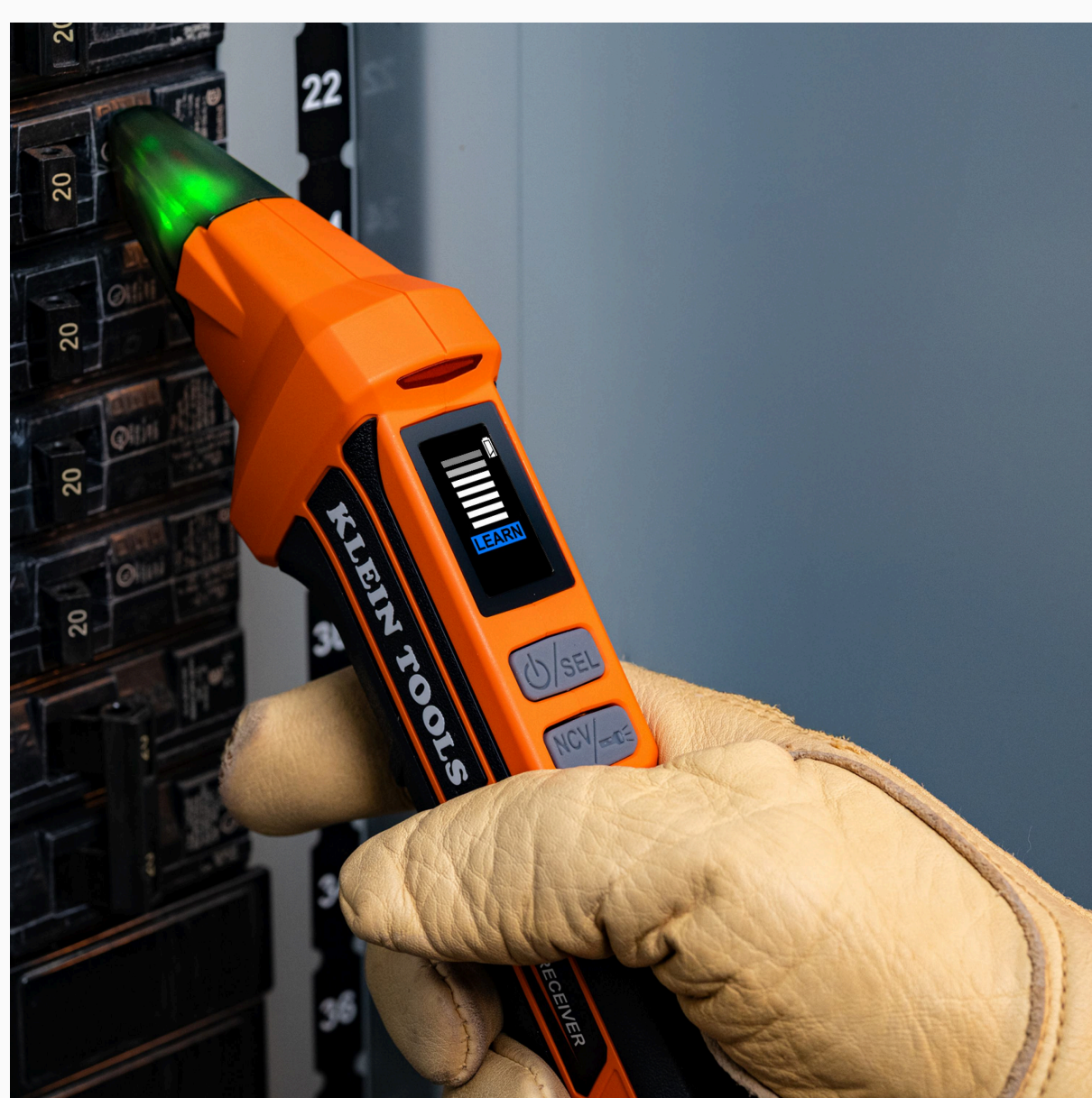
Circuit Breaker Finding
